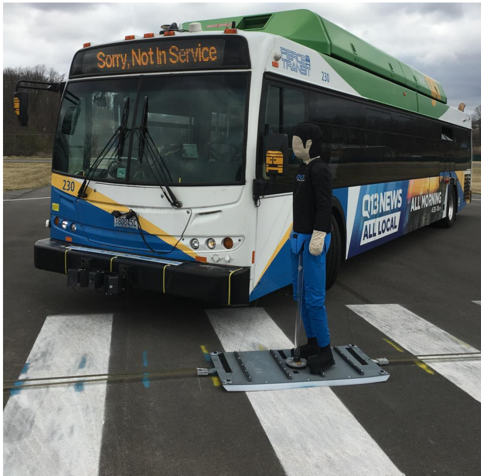
Figure 4 VRU Collision Avoidance Test Photo credit: VTTI
